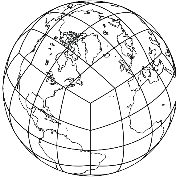
Fig. 2. Tiling the surface of the sphere with quadrilaterals. An inscribed cube is projected to the surface of the sphere. The faces of the cubed sphere are further subdivided to form a quadrilateral grid of the desired resolution. Coordinate lines from the gnomonic equal-angle projection are shown.
